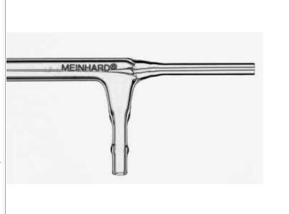
FOR LC-MS: the CIR-50-HK is designed to use 0.7 L/min of helium at 50 psig. A shortened liquid input allows for insertion of a fused silica LC column directly into the capillary of the nebulizer. Dead volume is virtually eliminated and there is no need for connective fittings.
