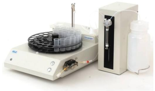
The tray configuration (number of positions, volumes of the vials) is free practicable. (standard: 89 x 8/4/2 ml, 53 x 16 ml, 36 x 30 ml, 18 x 50 ml), external positions (f.e. standards, control samples) are also practicable. Two different kinds of trays are recognized automatically.
