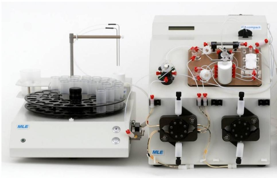
The **Universal Method Unit** joints the basic parameters of the water analysis
