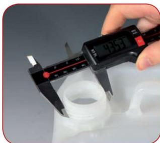
*Measuring of canister thread*
