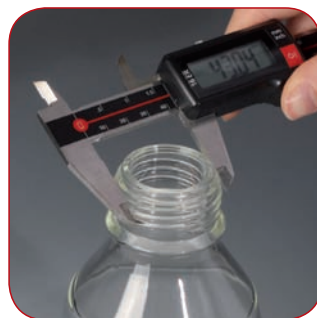
Measuring of bottle thread
