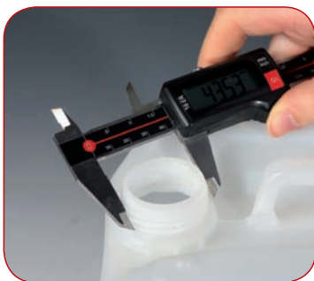
Measuring of canister thread
