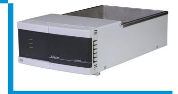
**Four-way gradient valve** is controlled from the pump ECP2010 and 2010H and gradient box ECB2004 must be ordered with the pump. Pumps have new sophisticated electronics which allows achieving precise **low-pressure gradient**, i.e. gradual **changes of mobile phase composition** by mixing **up to four liquids** at the pump's entry. It is also possible to predefine the percentage of composition when using the pump in isocratic mode. Gradient profile can be defined from computer or pump.
